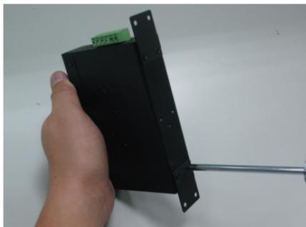
**Step 3:** Use the screws to screw the wall-mount plate on the Industrial Ethernet Extender.
