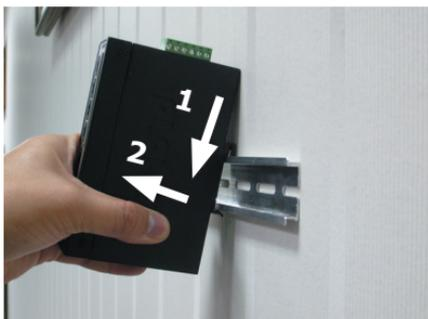
**Step 5:** Lightly pull out the bottom of DIN rail for removing it from the track.
