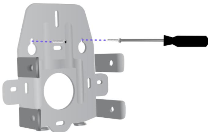
2. Connect the AP6-Pro-Outdoor to the Wall Mount using the 4 Screws with Washers and a Phillips screwdriver.
