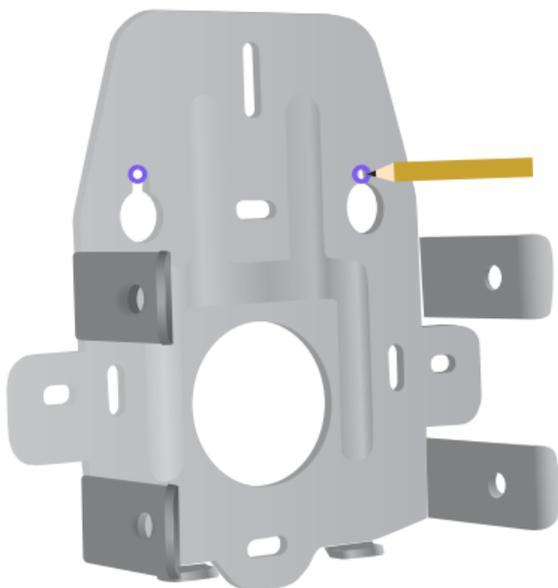
2. Use a 6 mm drill bit to drill the holes for the anchors.
