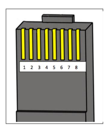
RJ45 plug pins are sorted by number, the sketch map is as shown above:
