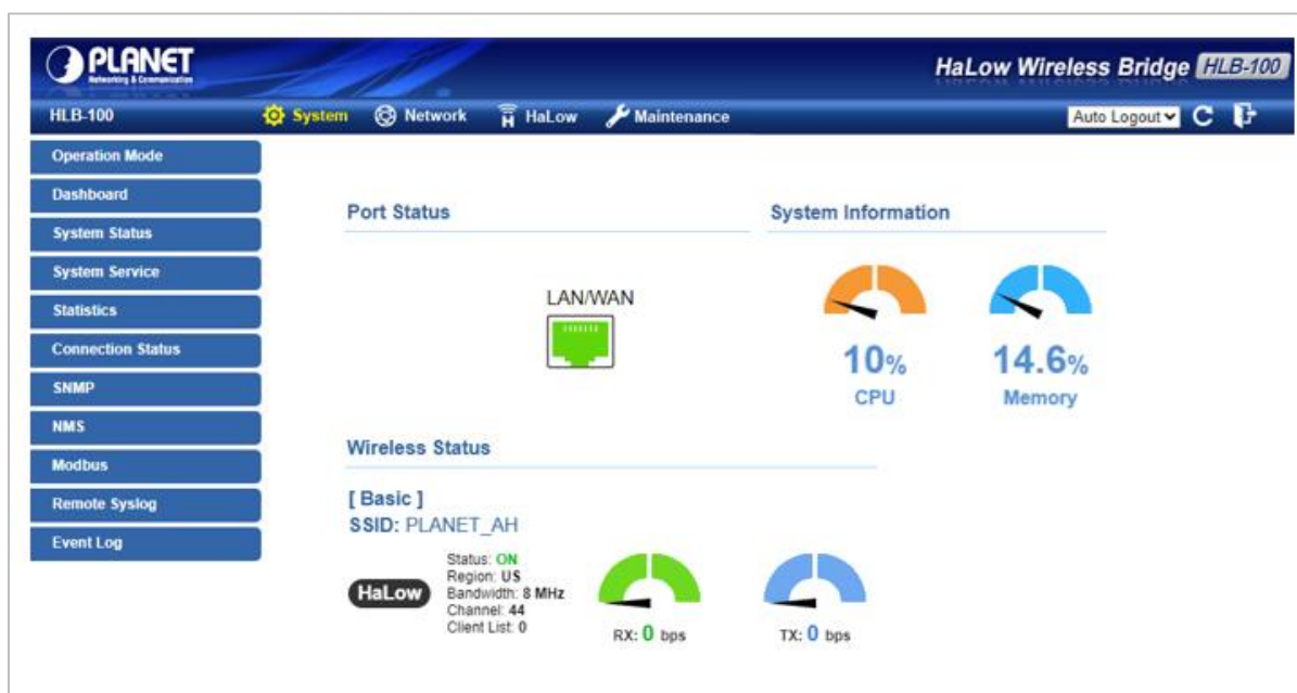
Figure 3-8: Web Main Screen of HaLow Network Device
