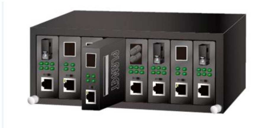
Figure 3-1: Insert HLB-100 into an available slot
