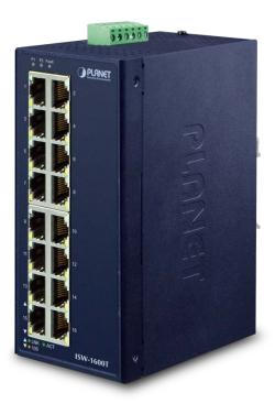
PLANET ISW-1600T **Industrial** high-density **16-port 10/100TX Fast Ethernet Switch** is equipped with a rugged IP30 metal case for stable operation in heavy industrial demanding environments. Thus, the ISW-1600T provides a high level of immunity against electromagnetic interference and heavy electrical surges which are usually found on plant floors or in curbside traffic control cabinets.
