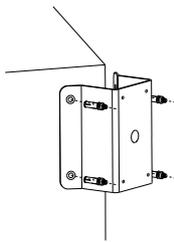
② Screw up and fix the bracket firmly
