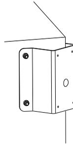
③ Complete the bracket installation and wiring for camera adoption
