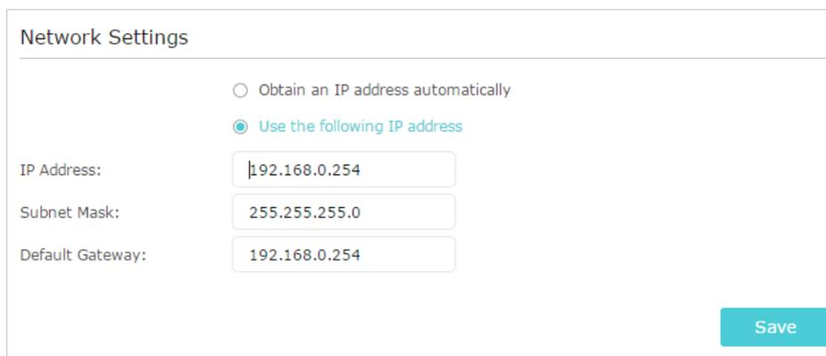
The screenshot shows a 'Network Settings' form. At the top, there are two radio buttons: 'Obtain an IP address automatically' (unselected) and 'Use the following IP address' (selected). Below this, there are three input fields: 'IP Address:' with the value '192.168.0.254', 'Subnet Mask:' with the value '255.255.255.0', and 'Default Gateway:' with the value '192.168.0.254'. A teal 'Save' button is located at the bottom right of the form.
