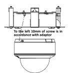
④ Insert the dome camera and bracket to the wall
