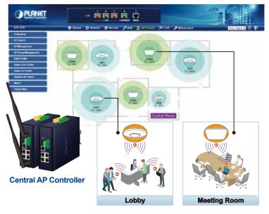
For example, to configure multiple smart APs of the same model, the IVR-300 allows clustering them to a managed group for unified management. According to requirements, wireless APs can be flexibly expanded or removed from a wireless AP group at any time. The AP cluster benefits bulk provision and bulk firmware upgrade through single entry point instead of having to configure settings in each of them separately.
