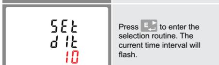
Use **M** and **P** buttons to choose the selection. Press **E** to confirm the setting and press **U/I** to return to the main set-up menu.
