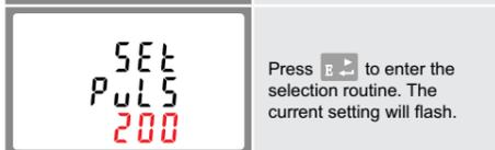
Use **M** and **P** buttons to choose pulse width. Press **E** to confirm the setting and press **U/I** to return to the main set-up menu.
