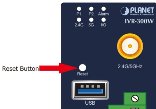
**Figure 5-1:** Reset Button of IVR-300 Series
