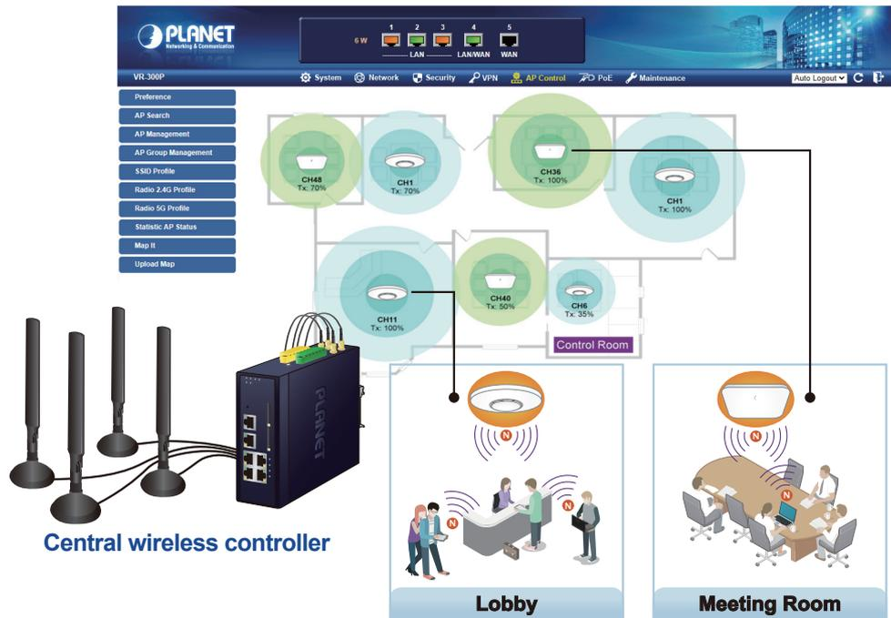
For example, to configure multiple Smart APs of the same model, the ICG-2515F-NR or ICG-2515FW-NR allow clustering them to a managed group for unified management. According to requirements, wireless APs can be flexibly expanded or removed from a wireless AP group at any time. The AP cluster benefits bulk provision and bulk firmware upgrade through single entry point instead of having to configure settings in each of them separately.
