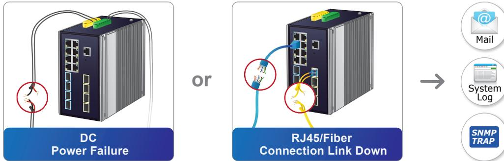
Digital Input and Digital Output for External Alarm
