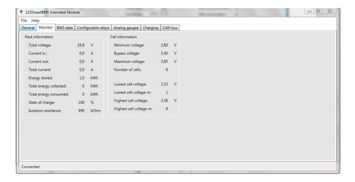
You can set the new values for used cells in the BMS data settings with also temperature protection and CAN ID address to broadcast the values on CAN bus.
