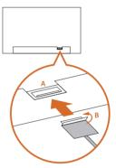
Connect the other end of the cable to the 40-pin eDP connector on the motherboard.
