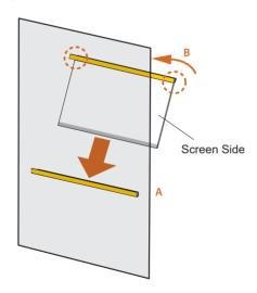
If you install them correctly, from the screen side, the silver mylar at the bottom of the eDP panel will be fully covered by the bracket.
