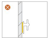
Install the other bracket on the top edge of the eDP panel. Make sure the screen is facing the same side as the sticker.
