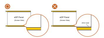
8. Peel off the paper liners from the rubber strips. Do not touch the adhesive surface. Paste the rubber strips closely along the edges of the eDP panel, so that the eDP panel is securely framed and won't shift or slide.
