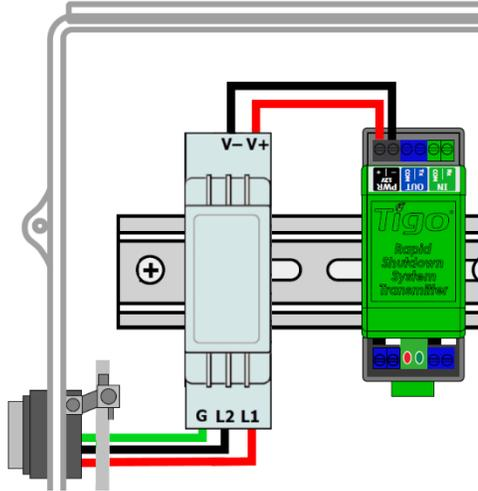
4. If connecting multiple transmitters, use parallel connections between all PWR terminals.
