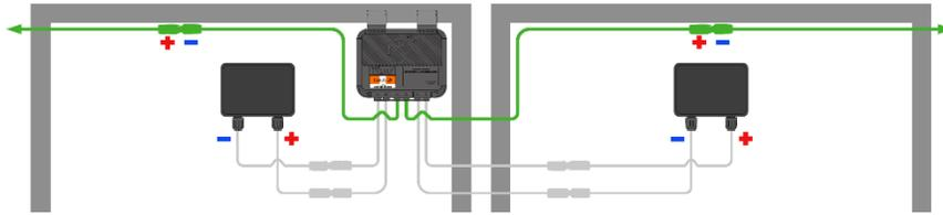
4. If connecting a TS4-A-2F to a single solar module, connect the unused second set of input cables.
