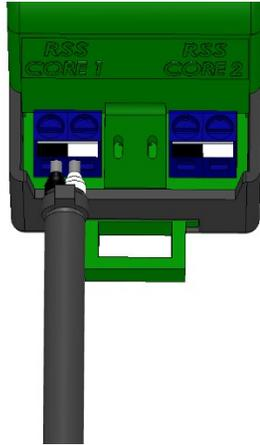
2. Insert the core wire with the black ferrule into the black terminal. Torque to 0.5 Nm.
