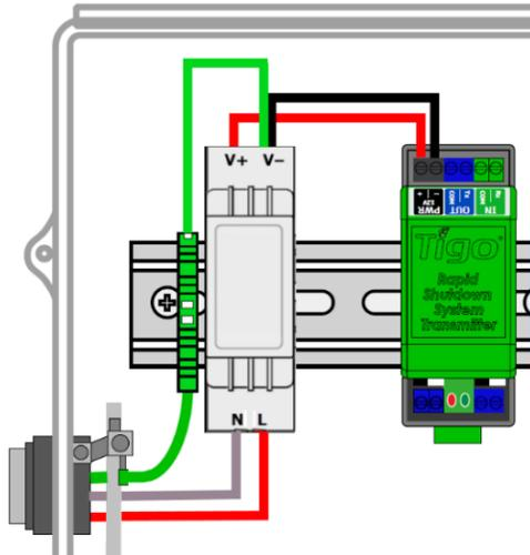
To connect a commercial 180-550 V/10 A power supply to a transmitter:
